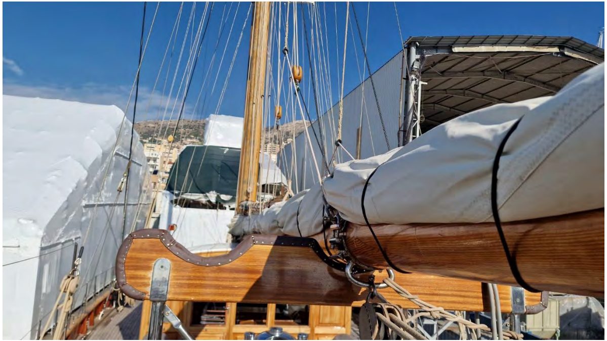
Photo 19 Resting post of main mast boom.
