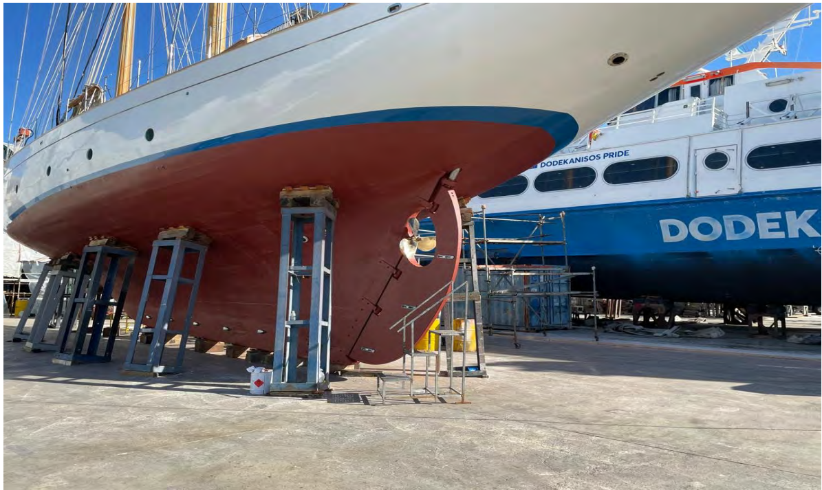
Photo 62 Stern view after completion of dry-docking works.
