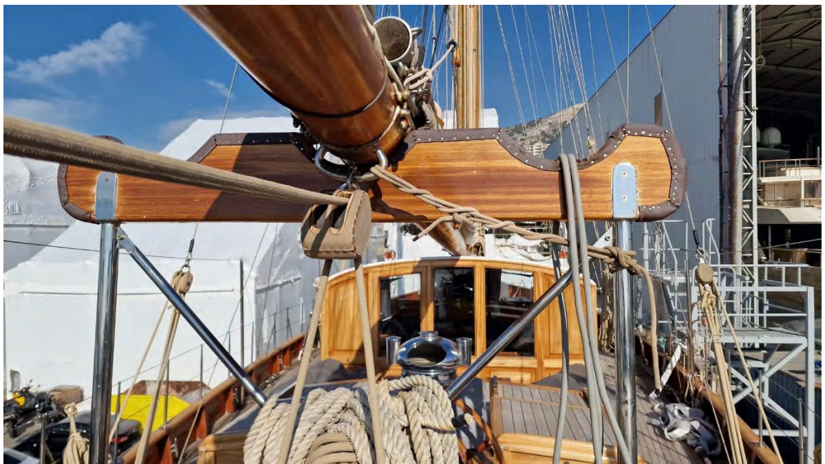
Photo 20 Special stainless steel structure for supporting the main mast boom.
