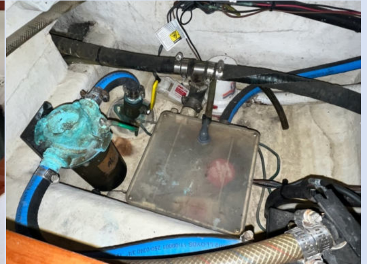
Portside head with Vacuflush toilet, MSD system, freshwater system, midship bilge pump, thru-hulls and sump pump appears in serviceable shape
