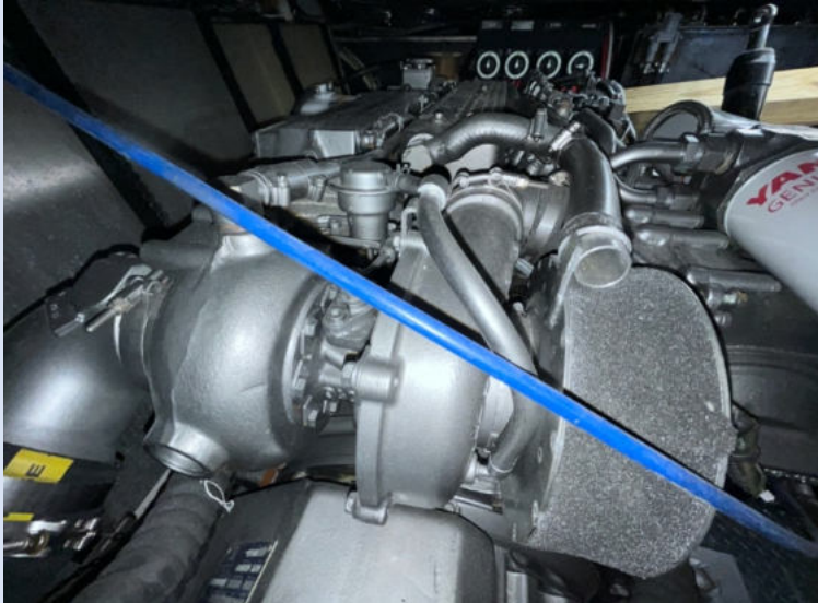
2x Yanmar 440HP diesel engine turbochargers and 8x motor mounts appear in functional condition without widespread surface rust or raw-water corrosion
