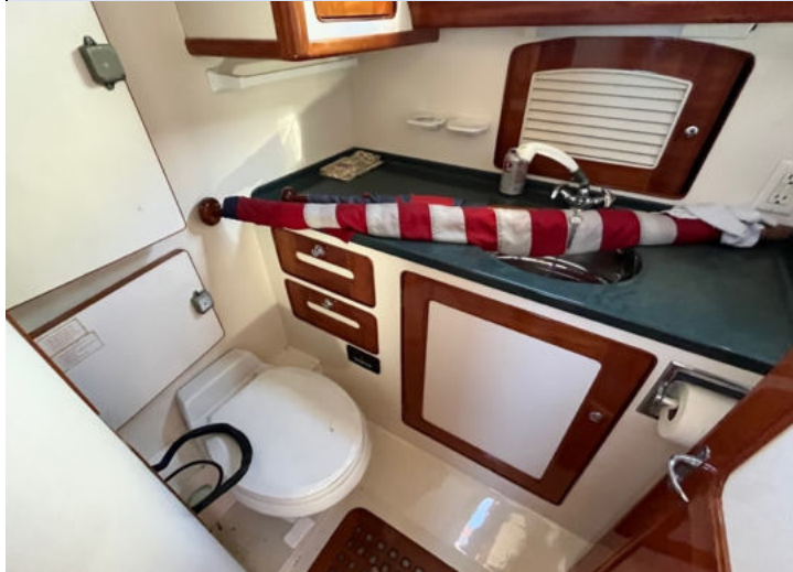
Portside head with Vacuflush toilet, MSD system, freshwater system, midship bilge pump, thru-hulls and sump pump appears in serviceable shape
