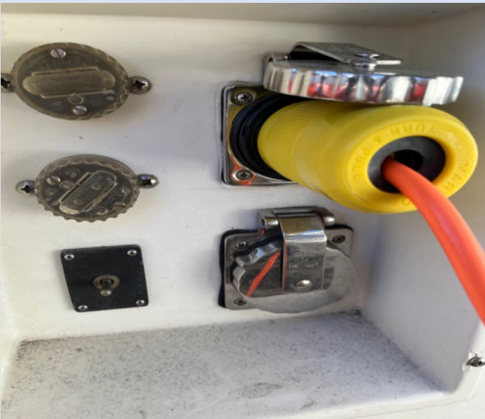
30A 125V shorepower dockside inlet and radar mast with Garmin radar antenna appears in serviceable condition
