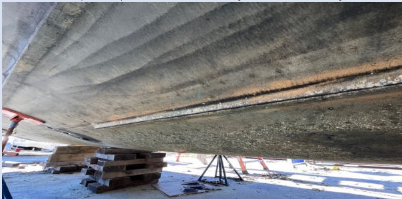
No grounding damage was reported to the hull bottom without osmotic blistering, FRP thruster tube and bow thruster appears in serviceable shape
