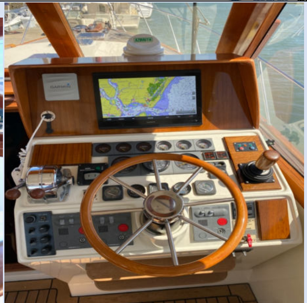
Aft cockpit is well-supported, structurally sound, teak and pilothouse helm station appears in serviceable shape with new Garmin GPS
