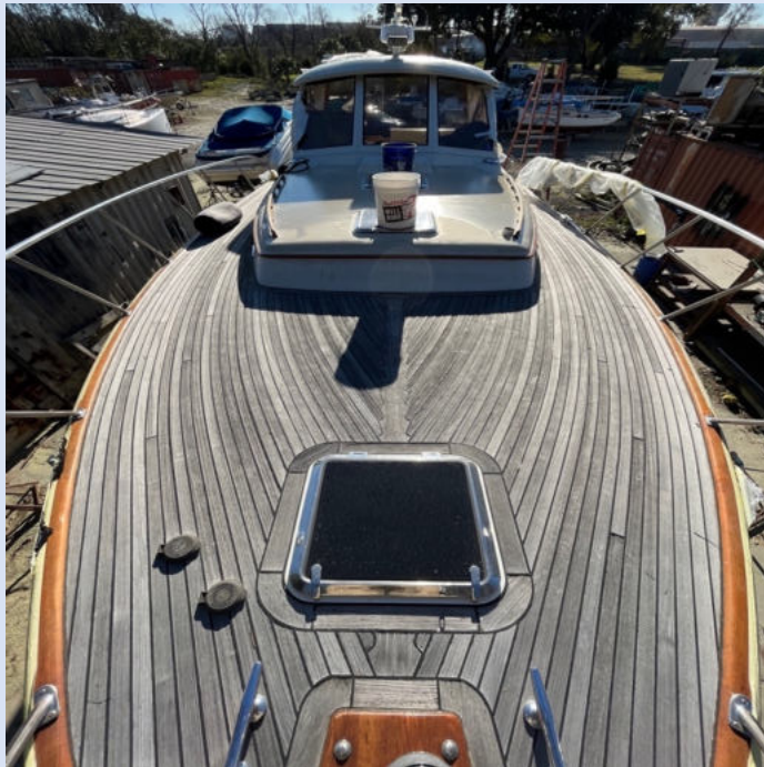
Teak foredeck, cabinhouse, deck hatches, handrails, lifelines, handrails, windshield, pilothouse and Maxwell anchor windlass appears in serviceable condition
