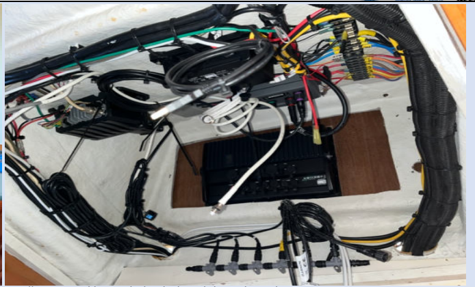
All systems appear in serviceable shape in the galley and wiring is well-supported beneath the dash and throughout the 44
