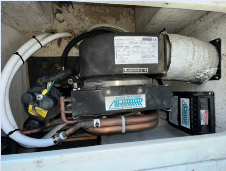
2x Dometic Marine Air Systems reverse cycle climate control units appear in serviceable shape and looking forward in the pilothouse
