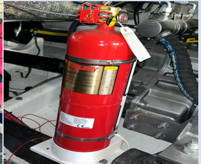
Rubber raw-water hoses, thru-hulls, seacocks, valves, sea-strainers, grounding wires, Racor diesel fuel-water separating filters & Fireboy suppression system is new
