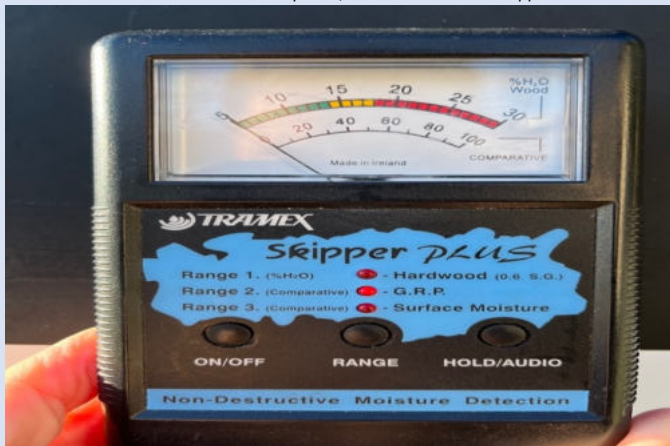
Normal, dry and acceptable Tramex moisture readings and FLIR thermal readings were taken throughout the hull exterior, on deck and structural support members
