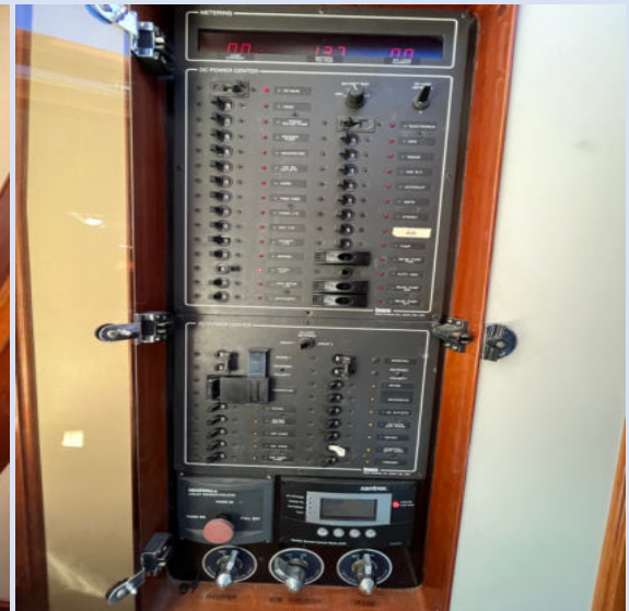
Looking forward in the main salon interior, AC and DC power distribution panel appears in serviceable shape and powers up
