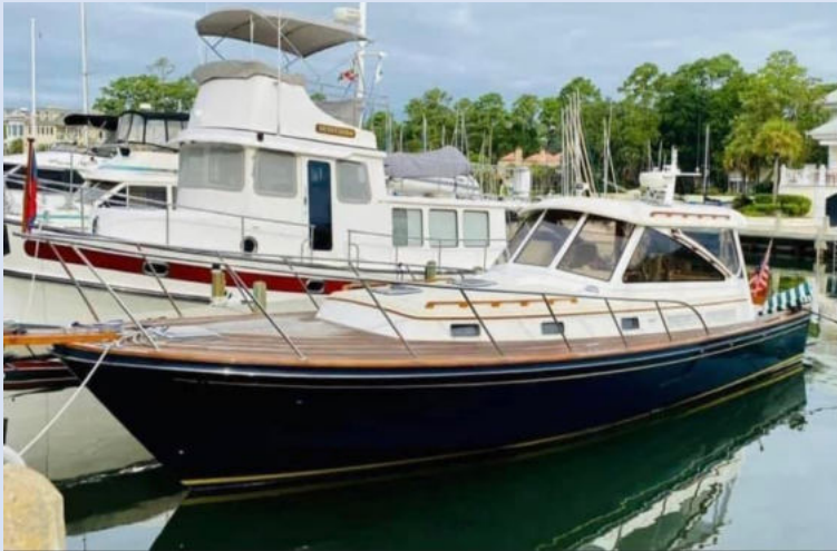
Port and starboard FRP topsides, hull bottom and keel appear in serviceable structural and cosmetic condition without delamination, water intrusion or soft-spots
