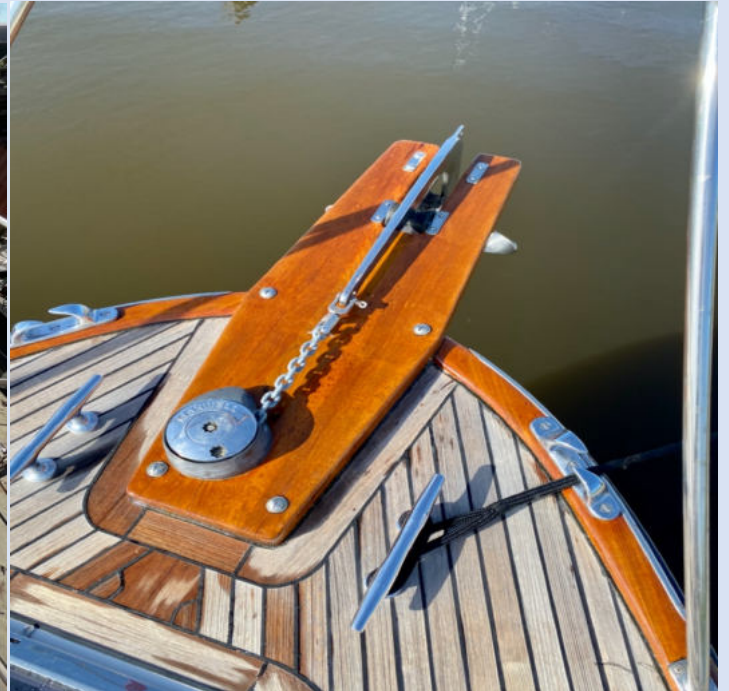
Teak foredeck, cabinhouse, deck hatches, handrails, lifelines, handrails, windshield, pilothouse and Maxwell anchor windlass appears in serviceable condition
