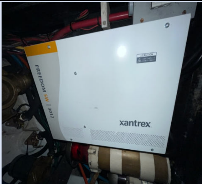
1x 12V DC Xantrex Freedom SW 3012 battery charger and inverter and new sea-strainer appears in bristol condition aboard the 44
