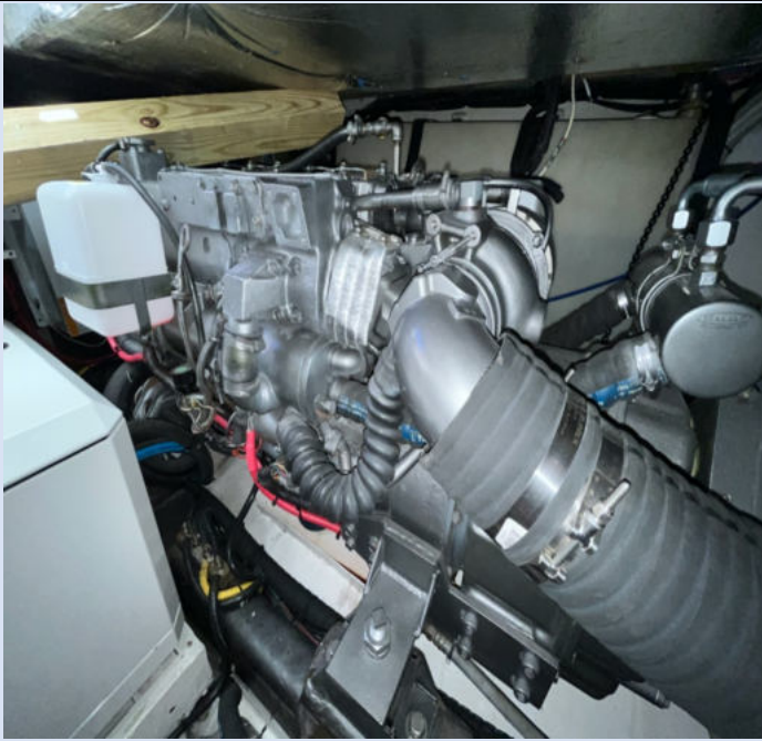
2x Yanmar 440HP diesel engines, 2x ZF Hurth marine transmissions and heat exchangers appear in serviceable condition without corrosion or critical wear
