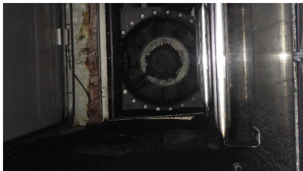
MAIN ENGINE ROOM EXHAUST FANS INSTALLED WITHOUT PROTECTIVE GUARD/SCREENS
