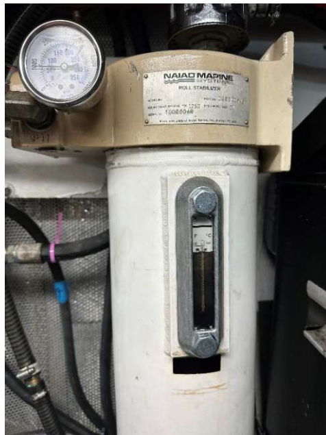
Stabilizer hydraulic fluid was changed after the last sea trial attempt and is Discolored again.
