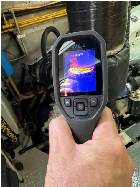
Exposed main Engine exhaust Hot spots
