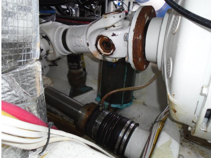
21. Engine drive shafts and shaft seal.
