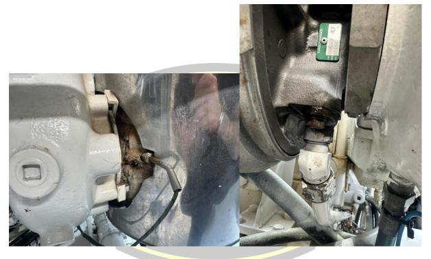
The exhaust heat wrap material you can see inside is burnt. This happens over long periods and is very normally but I would recommend replacement to stop the fiber particle material going inside the engine and clogging the air filter.
