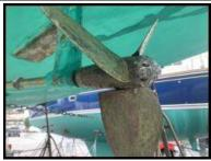
**Prop condition:** Prop is in good condition with no cracks, corrosion or bent, nicked or chipped blades.
