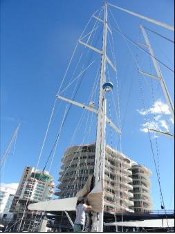
The mast was ascended and all mast and rigging fittings and components were inspected visually. The boom and components, all deck fittings, running rigging and lifelines were inspected visually.
