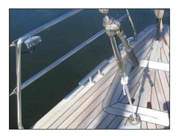
b. There is an extra piece of extrusion above the furling system on the rod.
