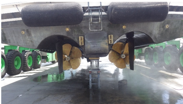
RUNNING GEAR -RUDDERS-PROPS
