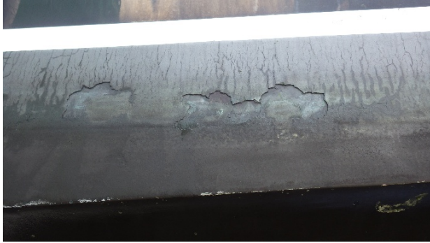
EXCESSIVE PAINT COATINGS (aka : MUD CRACKING) ALONG MOST OF THE WATERLINE
