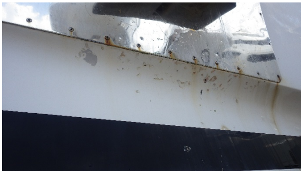
NUMEROUS CHIPS OF THE HULL SURFACE UNDER THE ANCHOR POCKETS
