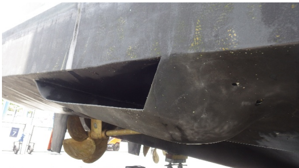
UNDERWATER MAIN ENGINE EXHAUST COWLING WITH INTERIOR PAINT COATINGS
