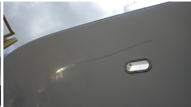
LARGE SCRATCH PORT SIDE HULL FWD. APPROXIAMATELY 3 FEET LONG
