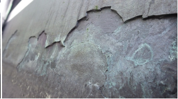
EXCESSIVE PAINT COATINGS (aka : MUD CRACKING) ALONG MOST OF THE WATERLINE
