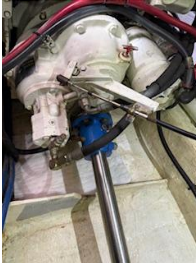
The starboard prop shaft coupling appears to have been recently replaced.
