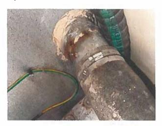
26. Corrosion and porosity were noted in the port engine exhaust riser. Repair or renew as deemed necessary.
