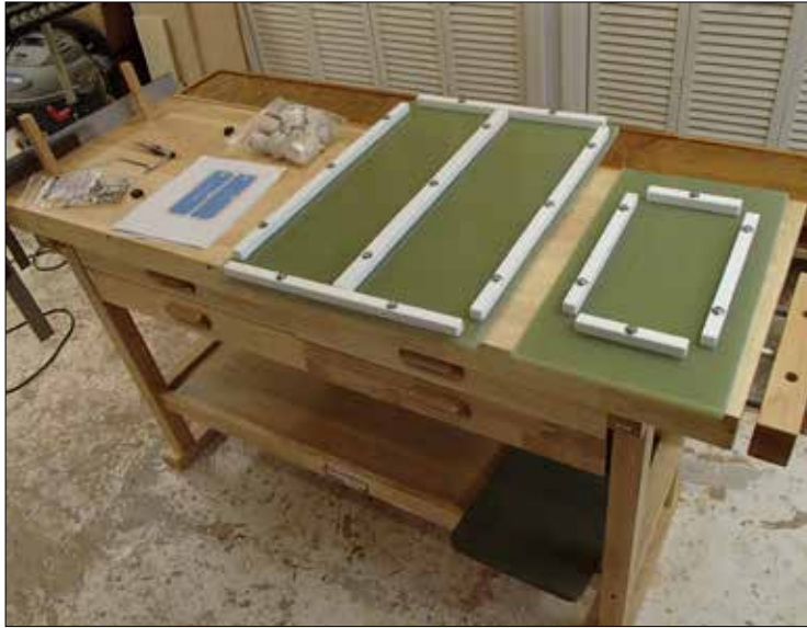
Left —Building a new base with brackets for the new lithium house bank, left, and for the smaller standard AGM starting battery. Considerations for housing the new system included adequate ventilation for temperature control around the new chargers but not the batteries themselves. Right —The author’s brother Greg Lenci unpacks one of the new lithium batteries dockside as the new system is installed.
