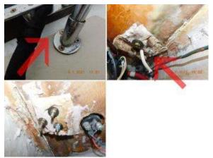
Stainless steel bow railing. Some stress cracking of the deck around base of port rear foot pad on the bow railing. Recommendation; have the deck repaired by a marine FRP technician and manufacture new backing pads that better form to the underside shape of the deck and replace the backing pads currently used to attach the bow railing to the deck. Stainless steel, well secured.
