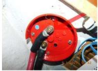
Rotary battery switch for the inverter supply does not have protection on the terminals. ABYC E 11.5.2.8 states; continuously energized parts, such as positive battery terminals and both ends of all wires connected thereto, shall be physically protected to prevent accidental short circuits. Protection shall cover all energized surfaces. Recommendation; cover battery terminals on the back side of the rotary switch.
