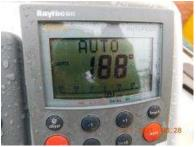
Mounted at pedestal instrument pod: Raymarine ST 6000. Powers up.
