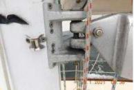
Aluminum - Well secured and no signs of abnormal wear. Extruded aluminum in good condition. Sparcraft carbon fiber boom vang.
