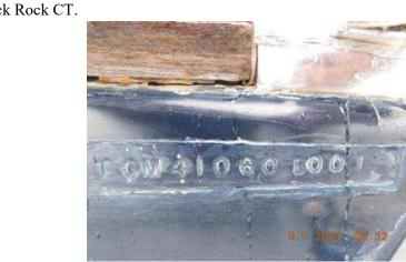
TCM 41060B001 A true digital photograph of the hull ID number of the referenced vessel is shown here and was found located on the transom. Fairport Yachts Fairport Harbor OH. February 2001. Fiberglass Auxiliary Sloop.
