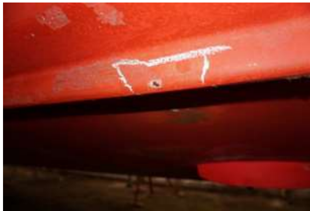
Figure 10.16 Flaw in epoxy/fiberglass on stab. bottom
