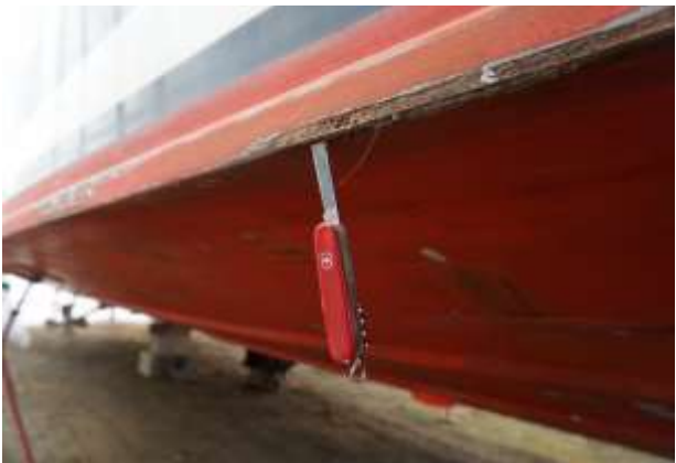
Figure 10.15 Crack in lifting rail/hull interface
