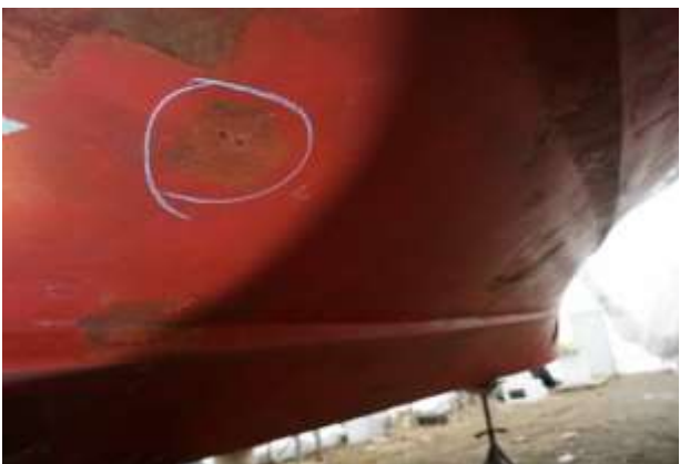
Figure 10.17 Circle marks flaws in epoxy/fiberglass on stb. bottom
