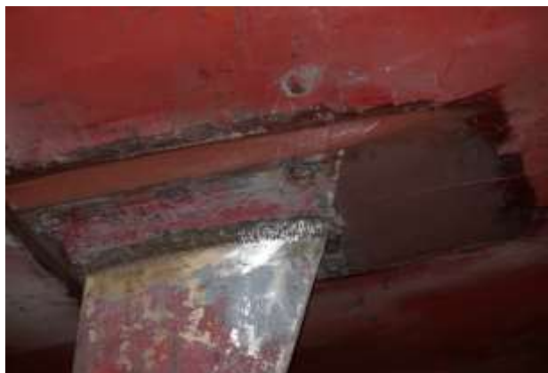
Figure 10.18 Fairing compound at hull & starboard strut interface
