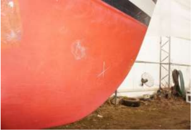
Figure 10.19 X marks area of small void/lifting fiberglass
