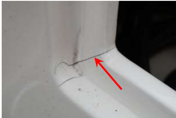
Figure 10.24 Crack in corner of cockpit storage locker
