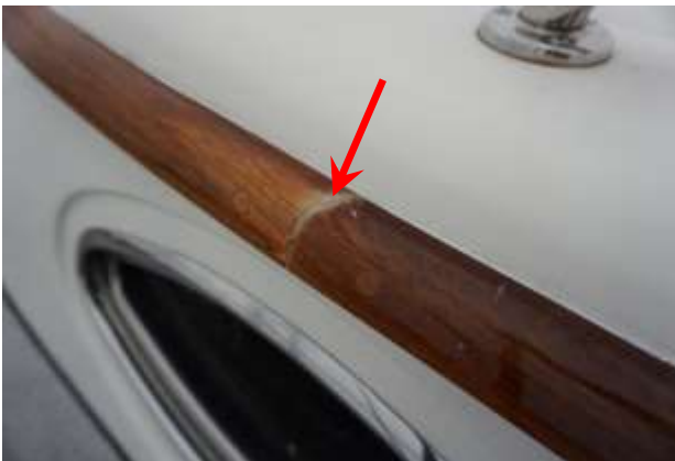
Figure 10.27 Imperfection in varnish
