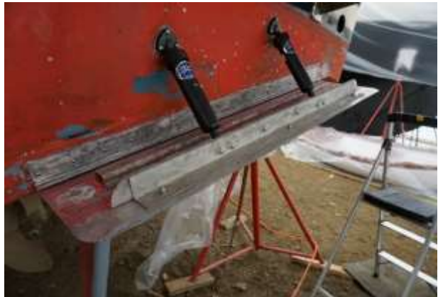
Figure 10.4 New trim tab & reinforcement assembly
