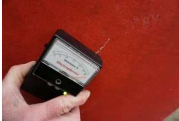
Figure 10.20 Elevated moisture on X mark on stb. bow
