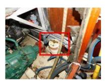
**Engine mounts and beds:** Engine mounts appear to be well secured to the support stringers.
