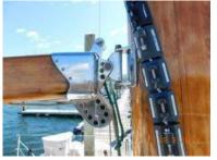
Masthead fittings: Anchor light, VHF antenna, Wind speed anemometer, Windex with tacking tabs.
