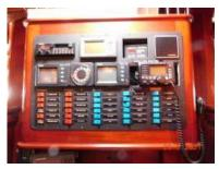
**Breaker(s)/fuse(s):** All D.C. circuits are adequately protected by branch or switched breakers.
