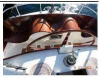
Sole: Scuppers/deck drain(s): Cabin entrance: FRP (fiber reinforced plastic) with applied in non skid.Yes. Drains are clear, hoses secure.Sliding custom entry hatches aft and amidships.
