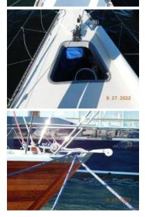
Stanchions/side rail(s):Stainless steel.Lifeline(s):Double stainless steel.Boarding gate:Port and starboard sides have boarding gates.
