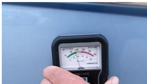
Acceptable Moisture Readings on the hull
