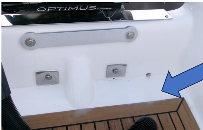
Stress Crack on the port Transom-No moisture
