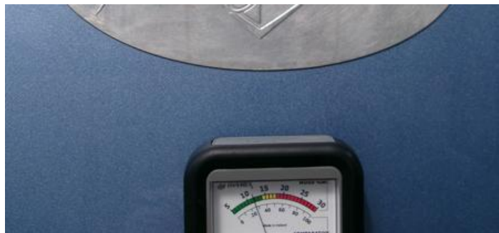
Acceptable Moisture Readings on the hull
