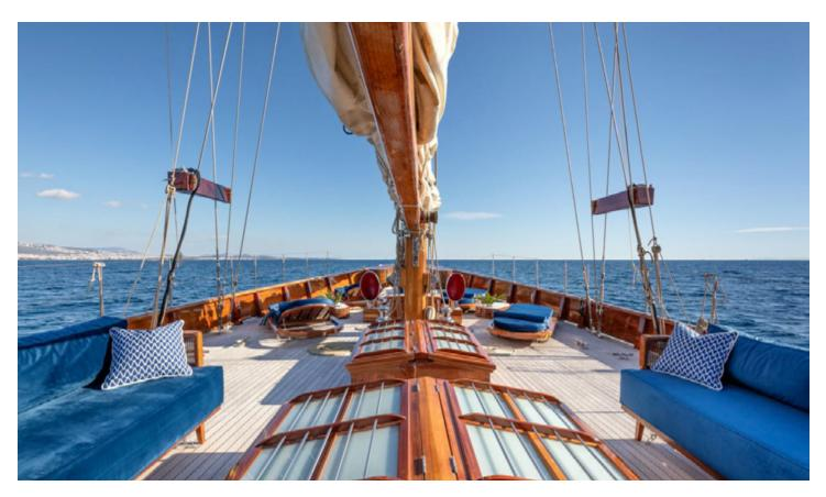
Weatherbird was built with an oak hull and teak superstructure and delivered in 1931 by French yard Chantier Navals de Normandie. Her classic lines were devised by Henri Rambaud while Victor Orloff developed the yacht's naval architecture.
