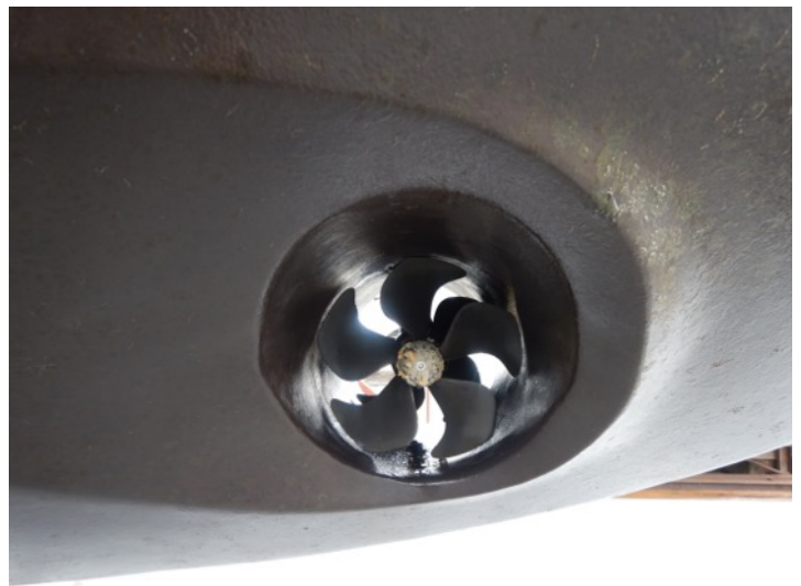
Electric Variable Speed SIDE-POWER Bow Thruster System
