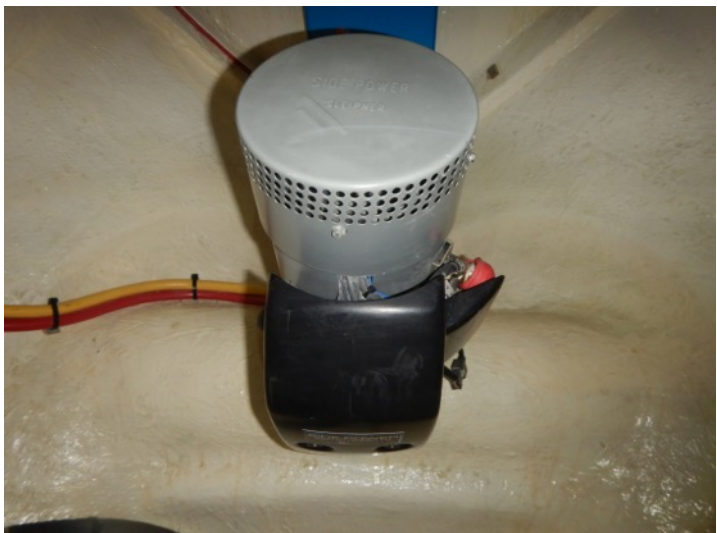
Electric Variable Speed SIDE-POWER Bow Thruster System
