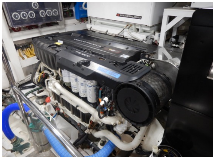
Twin Diesel Powered 900HP VOLVO PENTA Inboard Engines w/ VOLVO PENTA IPS Pod Drive Transmissions
