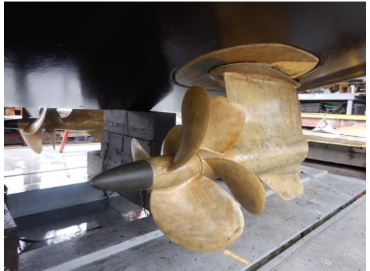
VOLVO PENTA IPS Pod Drive Transmissions w/ Counter Rotating Bronze Propellers
