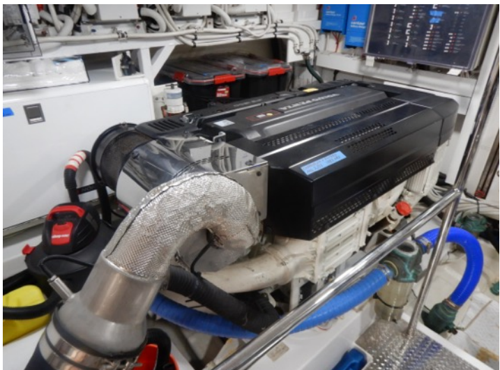
Twin Diesel Powered 900HP VOLVO PENTA Inboard Engines w/ VOLVO PENTA IPS Pod Drive Transmissions
