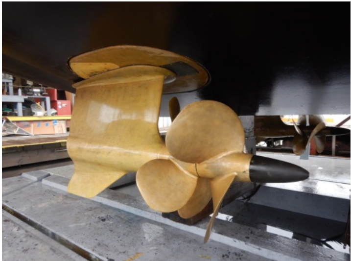
VOLVO PENTA IPS Pod Drive Transmissions w/ Counter Rotating Bronze Propellers
